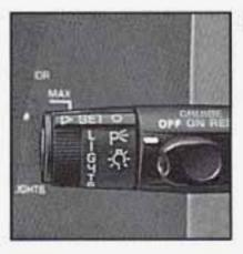
Move the Cruise switch to "OFF." (The "CRUISE" light will go out.)
