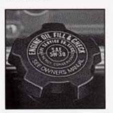
Turn off the engine and give the oil a few minutes to drain back into the oil pan.
