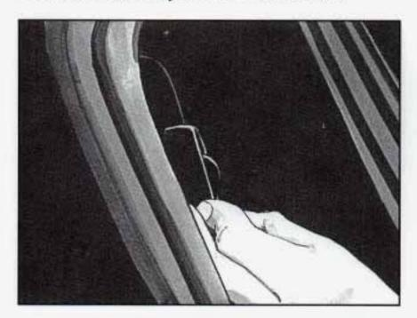
There is one guide for each outside passenger position in the rear seat. You will find them tucked in between the seat back and the interior body, about half-way down the edge of the seat back. Here is how you should install the comfort guide on the shoulder belts:
