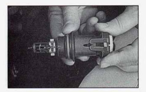
Remove the wire connector from the bulb by lifting the lock tab and pulling it away from the plastic base. Replace the bulb. Reverse the procedures to reinstall the headlamp bulb.
