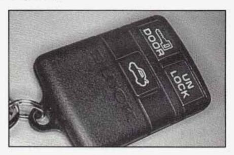
If your Buick has this option, you can lock and unlock your doors or unlock your trunk from up to 30 feet (9 m) away using the key chain transmitter supplied with your vehicle.
