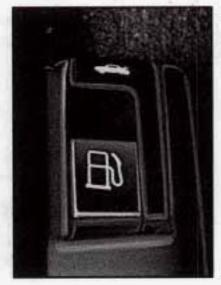
Pull up on the release lever to unlatch the fuel door. It is located on the floor to the left of the driver's seat.
