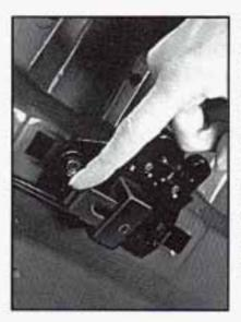
The lockout switch, located on the inside of the trunk lid, allows you to disable the remote trunk release inside the passenger compartment. With the lockout control in the OFF position, you can use the remote trunk release. You must use the trunk key when the lockout control is in the ON position.
