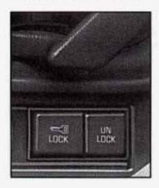
Press the power door lock switch to lock or unlock all the doors at once.
