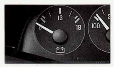
This gage shows the voltage in the electrical system.
