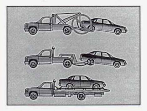
Use wheel lift or car carrier equipment. Additional ramping may be required for the car carrier equipment. Use safety chains and wheel straps.
