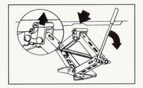
Raise the vehicle by rotating the wheel wrench clockwise. Raise the vehicle far enough off the ground so there is enough room for the spare tire to fit.
