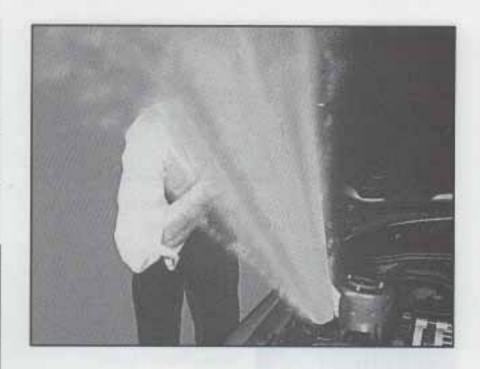
Adding only plain water to your cooling system can be dangerous. Plain water, or some other liquid like alcohol, can boil before the proper coolant mix will. Your vehicle's coolant warning system is set for the proper coolant mix. With plain water or the wrong mix, your engine could get too hot but you wouldn't get the overheat warning. Your engine could catch fire and you or others could be burned. Use a 50/50 mix of clean water and a proper antifreeze.
