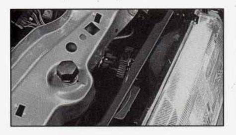
Raise the hood and locate the headlamp bulb retainers.
