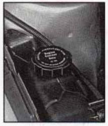
Then replace the pressure cap. Be sure the pressure cap is tight.
