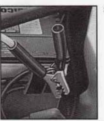
Now connect the black negative (-) cable to the good battery's negative (-) terminal. Don't let the other end touch anything until the next step. The other end of the negative cable <u>doesn't</u> go to the dead battery. It goes to a heavy unpainted metal part on the engine of the vehicle with the dead battery.
