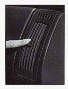
Adjust the direction of air flow by moving the louvered vents.
