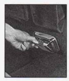
To remove the rear ashtray for cleaning, press down on the snuffer as you pull the ashtray down and out.
