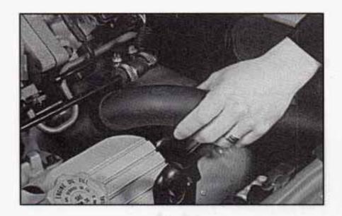
With the coolant surge tank pressure cap off, start the engine and let it run until you can feel the upper radiator hose getting hot. Watch out for the engine fan. By this time, the coolant level inside the coolant surge tank may be lower. If the level is lower, add more of the proper mix to the coolant surge tank until the level reaches the split line formed by the black and white part of the tank.
