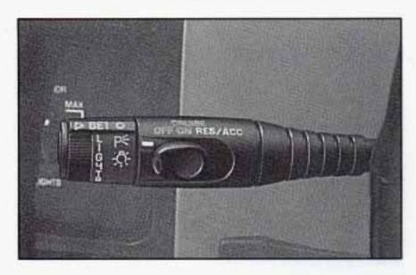
Move the Cruise switch from "ON" to "RES/ACC" Hold it there until you get up to the speed you want, and then release the switch. To increase your speed in very small amounts, move the switch to "RES/ACC" for less than half a second and then release it. Each time you do this, your vehicle will go about 1 mph (1.6 km/h) faster.
