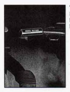
To release the parking brake: Hold the regular brake pedal down. Pull the brake release lever.
