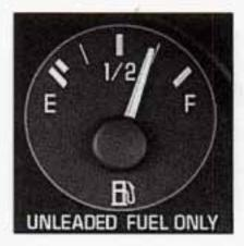
Your fuel gage shows how much fuel is in your tank. It works only when the engine is on. When the indicator nears "E," you still have a little fuel left. You need to get more right away. Here are four concerns some owners have had about the fuel gage. All these situations are normal and indicate nothing wrong with the fuel gage.
