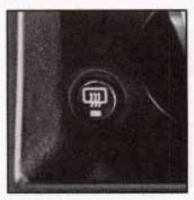
The lines you see on the rear window warm the glass. Press the button to start warming your window. Pressing the button again will shut it off.
