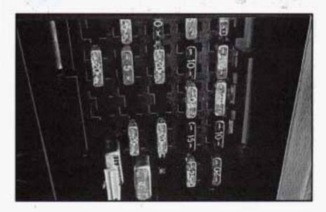
The fuse panel is to the left of the steering column, near the parking brake release lever. Pull the cover down to access the fuses.
