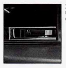
From the inside: To lock the door, slide the lock control rearward.
