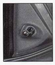
To adjust the left outside mirror, rotate the knob located on the driver's door.
