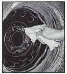
Remove any rust or dirt from the wheel bolts, mounting surfaces or spare wheel.
