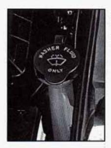
Open the cap labeled "WASHER FLUID ONLY." Add washer fluid until the bottle is full.
