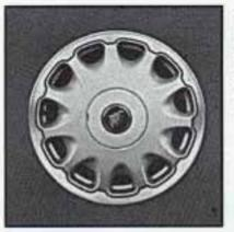
To remove this wheel cover use the flat end of the wheel wrench. Take the small cover off to access the wheel nuts.
