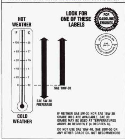
As shown in the chart, SAE 5W-30 is best for your vehicle. However, you can use SAE 10W-30 if it's going to be 0°F (-18°C) or above. These numbers on an oil container show its viscosity, or thickness. Do not use other viscosity oils, such as SAE 10W-40 or SAE 20W-50.
