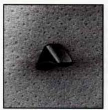
To fold a front seatback forward, push the seatback toward the rear as you lift this latch. Then the seatback will fold forward. The latch must be down for the seat to work properly.
