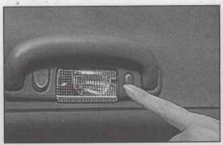
The rear seat reading lights are turned on by pressing the switch next to the light above the rear doors.
