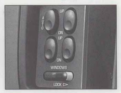
If your car has this option, the controls are near each window. Your driver's window has an express-down feature. Quickly press and release the AUTO switch and the driver's window will open a small amount. If the AUTO switch is pressed for more than a few seconds, the window will go all the way down. To stop a power window while it is lowering, press and release the
