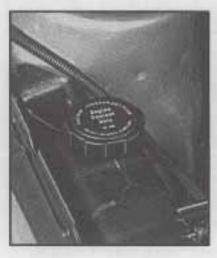
The surge tank is located on the passenger's side of the engine compartment.
