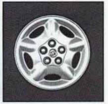
Remove either of these wheel covers by using the flat end of the wheel wrench. Pry along the edge of the wheel cover until it comes off. Be careful; the rim edges may be sharp. Don't try to remove it with your bare hands.
