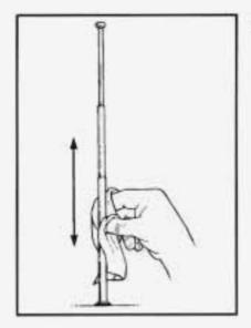
Wipe cloth over the mast sections, removing any dirt.
