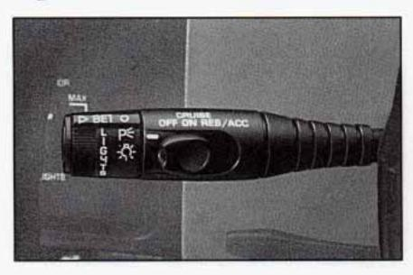
The headlight switch is located on the control left of the steering column.
