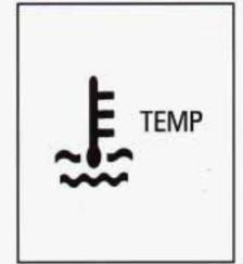
This light tells you that your engine coolant has overheated or your radiator cooling fan is not working. If you have been operating your vehicle under normal driving conditions, you should pull off the road, stop your vehicle and turn off the engine as soon as possible.
