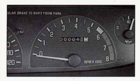
The tachometer tells you how fast the engine is running. It displays engine speed in hundreds of revolutions per minute (RPM).
