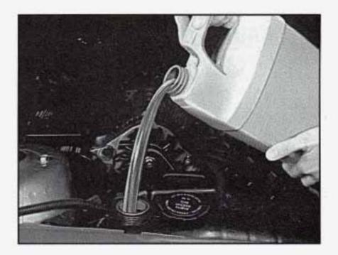
Fill the coolant surge tank with the proper mix, up to "FULL COLD" or just above the small cylinder at the base of the opening.
