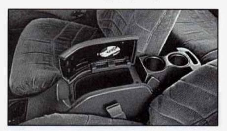
The console between the front seats has rear seat cupholders that when pulled up and rotated backward can be used. There is also a small tissue holder in the cover.
