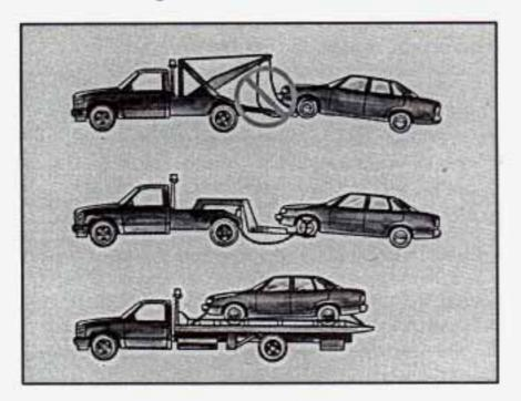
Use wheel lift or car carrier equipment. Additional ramping may be required for the car carrier equipment. Use safety chains and wheel straps.
