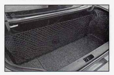
Your vehicle may have a convenience net. You'll see it just inside the back wall of the trunk. Put small loads, like grocery bags, behind the net. It can help keep them from falling over during sharp turns or quick starts and stops. The net isn't for larger, heavier loads. Store them in the trunk as far forward as you can. You can unhook the net so that it will lie flat when you're not using it.
