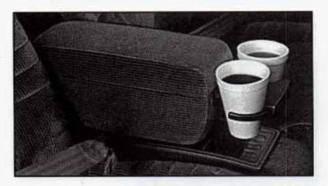
The armrest between the front seats opens into a storage area. To open it, press the lever at the front edge. Inside are cupholders which can be rotated forward for use with the cover closed. There is a storage area for cassette tapes, compact discs or other small items.
