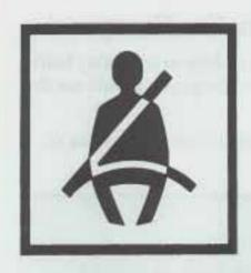
This figure lights up as a reminder to buckle up. (See "Safety Belt Warning Light" in the Index.)
