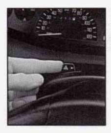
Move the switch to the right to make your front and rear turn signal lights flash on and off.
