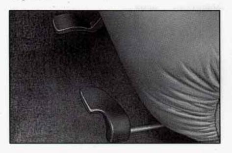
If you have this option, you have two levers under the front edge of the seat. The lever near the outer side of the seat unlocks the seat allowing it to slide forward and back. The lever near the center allows you to tilt the seat up and down.
