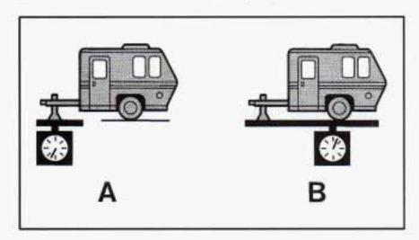
The trailer tongue (A) should weigh 10% of the total loaded trailer weight (B).
