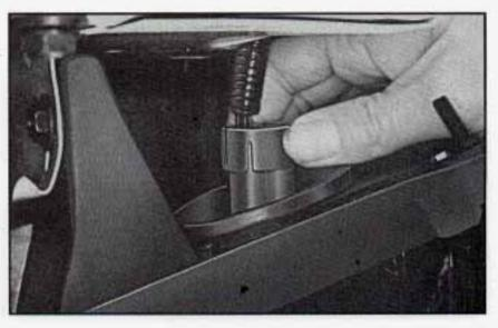
Pull the bulb/socket straight out from the access cover.
