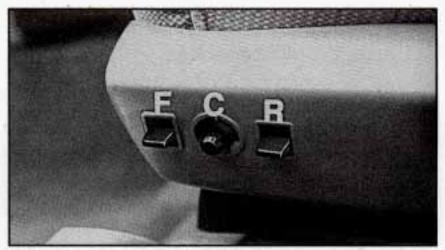
The power seat control is located on the side of the seat.
